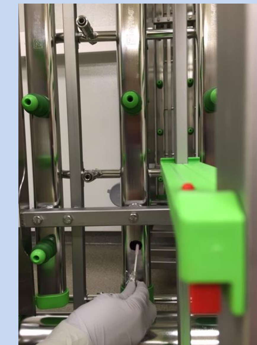
Figure 5. Swabbing of rack plenum for PCR analysis to confirm sterility at beginning of study.
