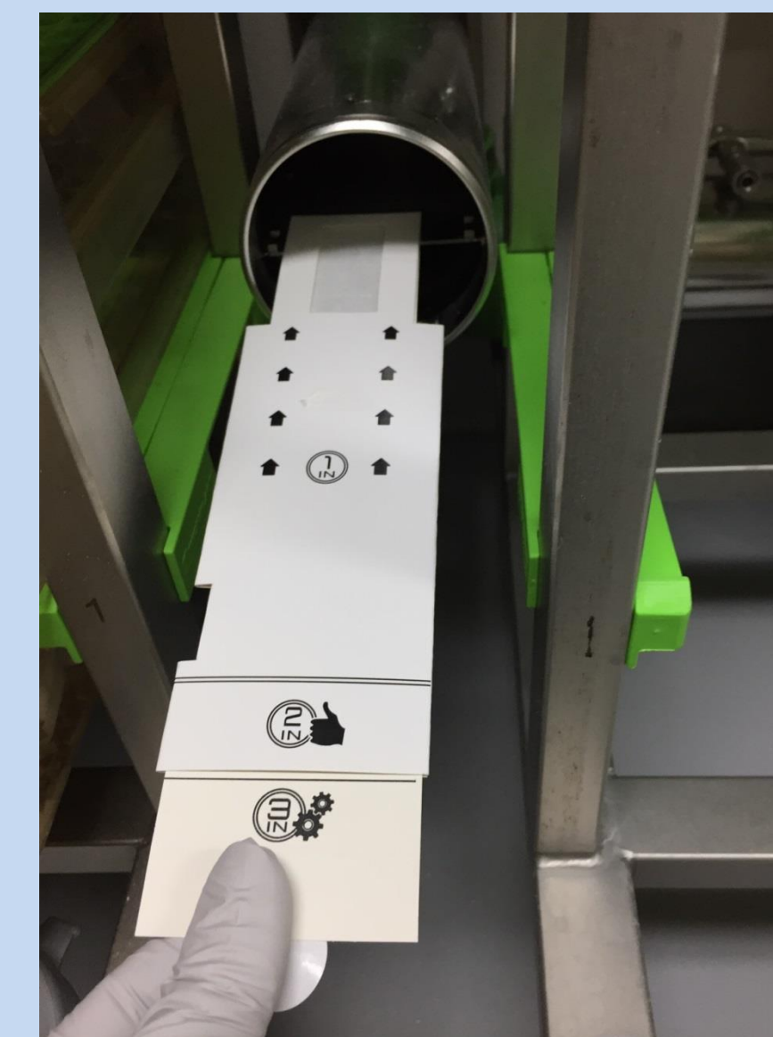
Figure 4. Interceptor being placed into the plenum attachment.
