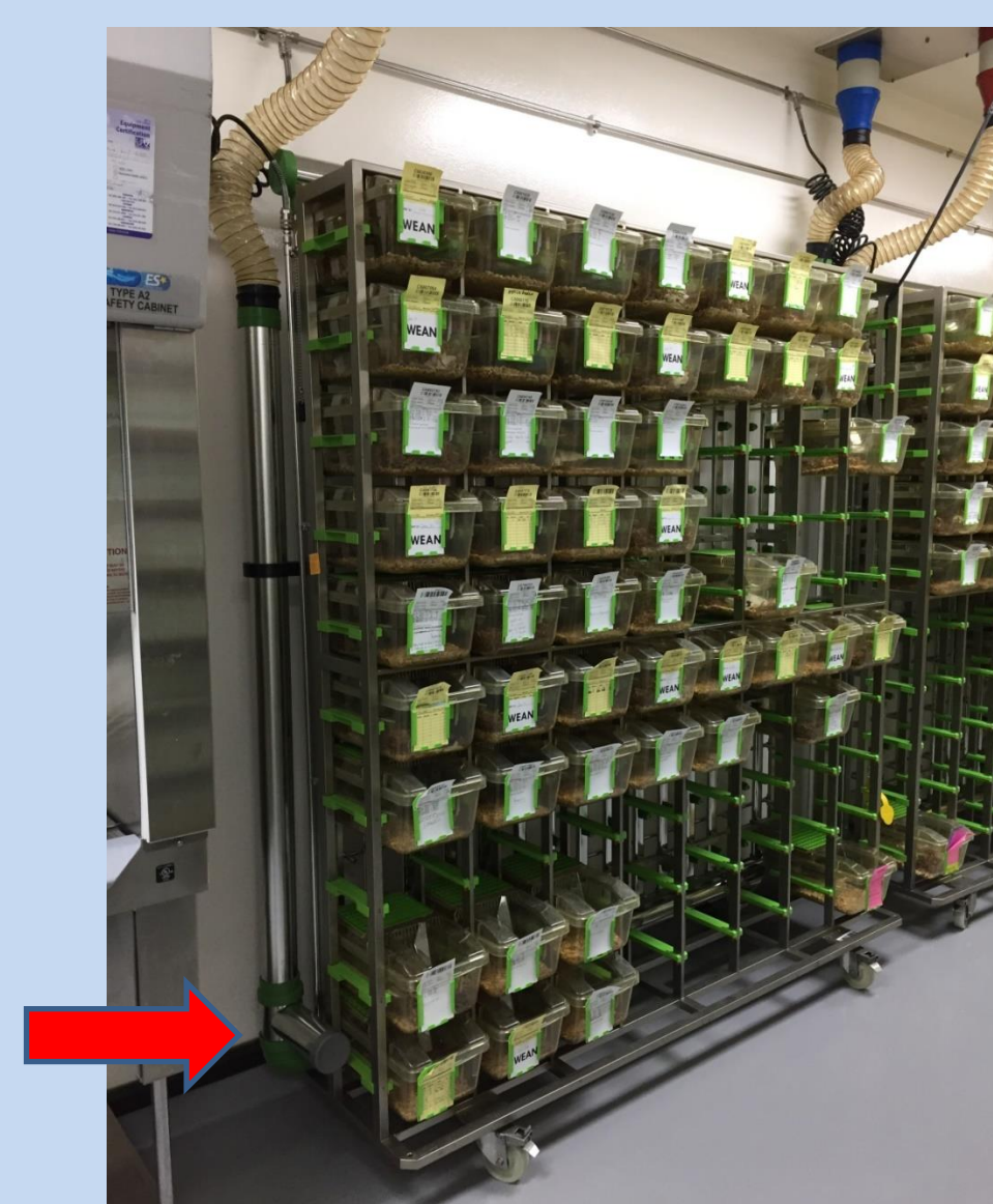
Figure 1. Two racks were fitted with a prototype plenum attachment to perform EAD testing (red arrow).
